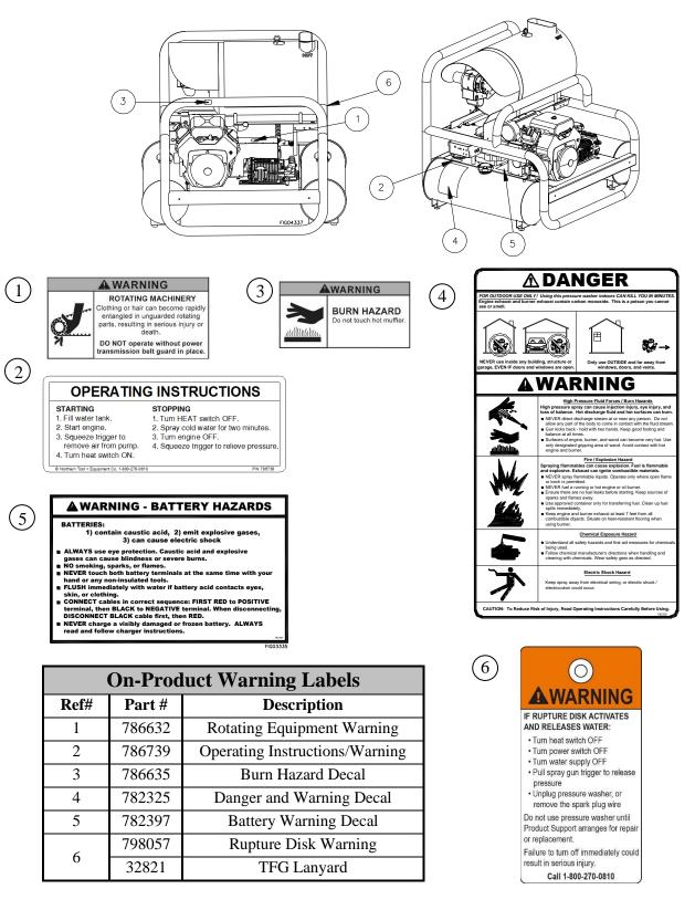
Always make sure safety labels are in place and in good condition. If a safety label is missing or not legible, order new labels or unsafe operation could result. To order replacement safety labels, call Northstar Product Support at 1-800-270-0810.
