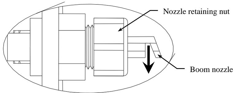
**IMPORTANT:** Make sure broadcast nozzle is oriented to spray straight back, parallel with the ground, before you start. An incorrectly positioned broadcast nozzle may spray chemicals on you or others.
