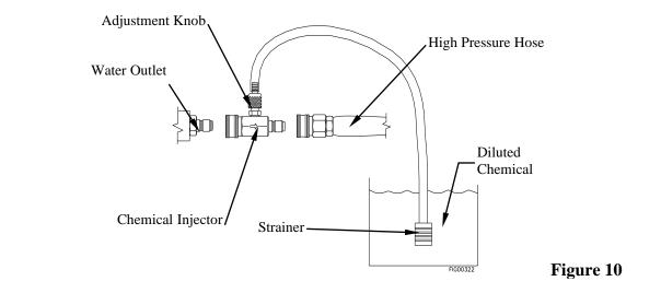
4. Submerge the suction strainer connected to the braided chemical hose into a bucket containing the chemical solution. See Figure 10.
